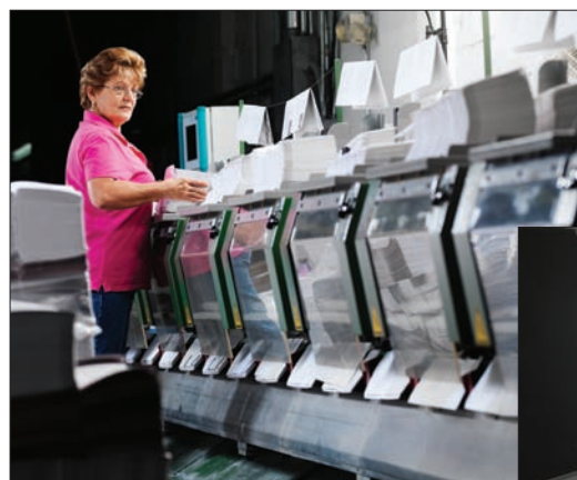
Clockwise, from the top: An employee loads the pockets of Solo's Muller Martini Bravo-T saddlestitcher. Right, work from the Fuji Sumo platesetter is inspected. Below, the pride and joy at Solo Printing is its new Komori System 38S heatset web press.
